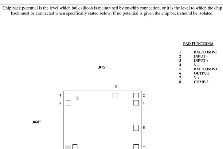
Top Material: Al Backside Material: Si Bond Pad Size: .004" min. Backside Potential: V-
